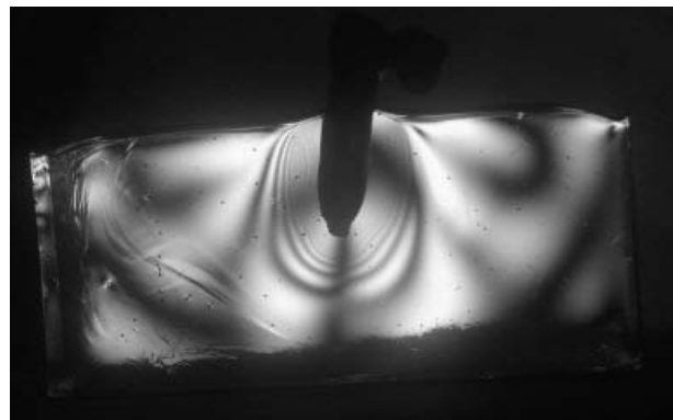
Figure 5. View of tensions at polariscope for probe 3 (optic zoom).
