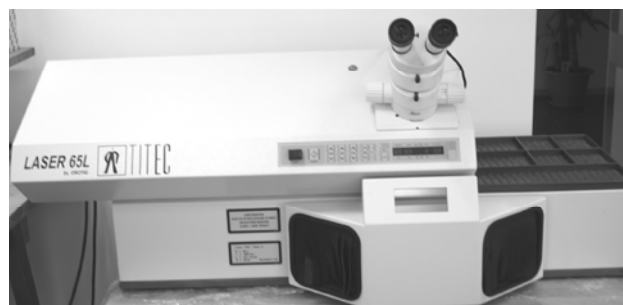
Figure 4. The Nd-Yag Laser equipment (Orotig) used for the weldings.
