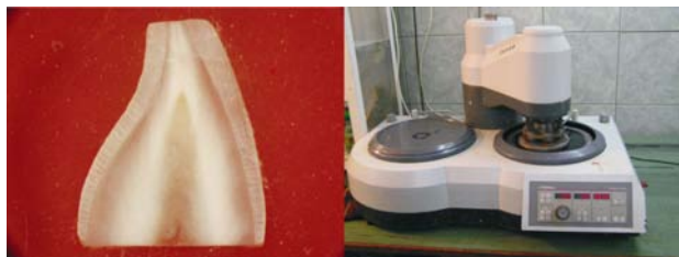
Figure 1. The sample preparation for measuring the enamel microhardness.
