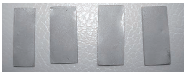
Figure 5. Casted plates after sandblasting and finishing.
