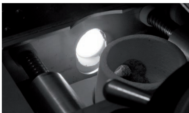
Figure 3. Casting of the Co-Cr alloy.
