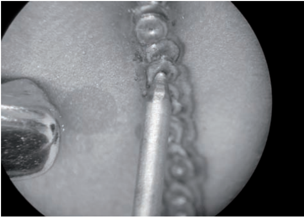
Figure 6. Microplasma welding of the plates.
