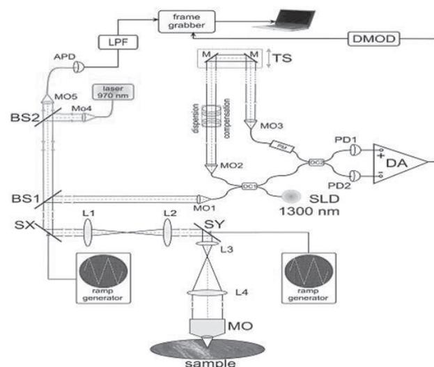
**Figure 3.** Experimental set-up used for eFOCT, including a super luminescent diode (SLD) emitting at 1300 nm with a bandwidth of 65 nm (DC1 and DC2 – directional couplers; MO1 and MO2 – arms of the interferometer; BS1 - dichroic beam-splitter; SX and SY - galvanometer scanners; DA - balanced photodetection unit; TS - computer driven translation stage)
